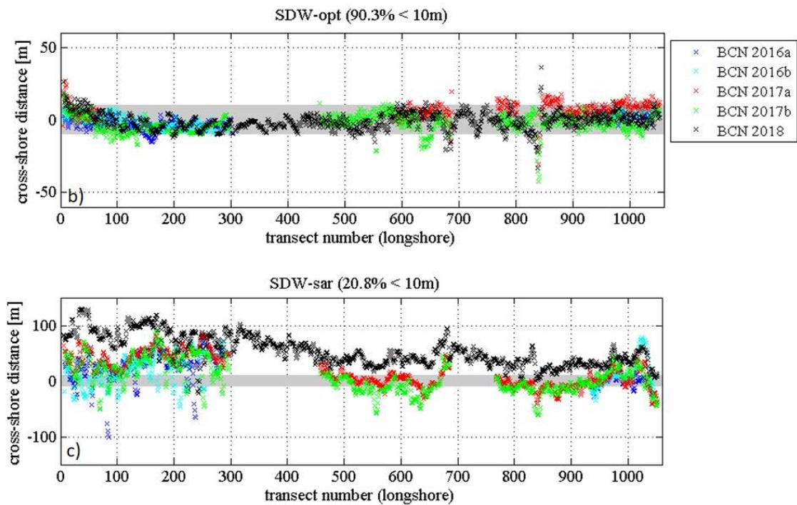
**Figure 15: Cross-shore transects along the coast from El Prat to Ginesta - Barcelona (a) and the distance between waterlines obtained from in-situ measurements and SDW-opt (b) and SDW-sar (c). The gray area indicates the range between  $\pm 10$  m.**
