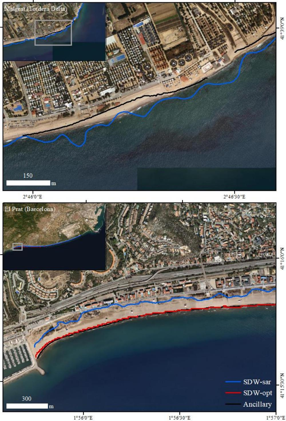
**Figure 16: Examples of waterlines obtained from in-situ measurements, SDW-sar and SDW-opt in Malgrat (upper map) and Barcelona (lower map).**
