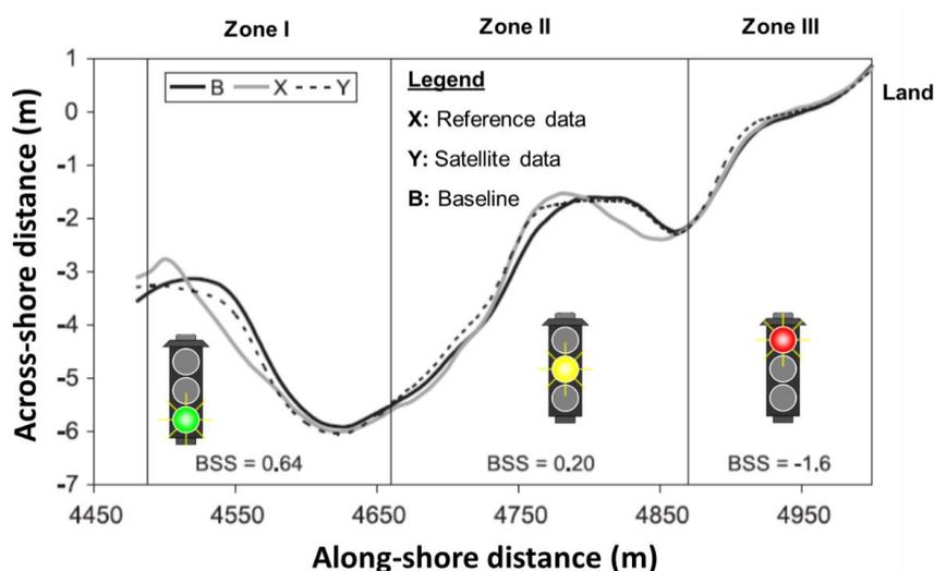
**Figure 3: Illustration of how the BSS will inform the skills of shoreline changes from space. End-uses will assess the adequacy of the skill for each application and site using a simple traffic light colour scheme.**
