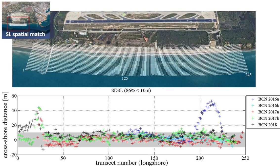
**Figure 13: Cross-shore transects displaced in the area where the shorelines match (upper panel) and distance verified between measured and satellite-based shorelines in each of those transects. The gray area indicates the range between  $\pm 10$  m.**
