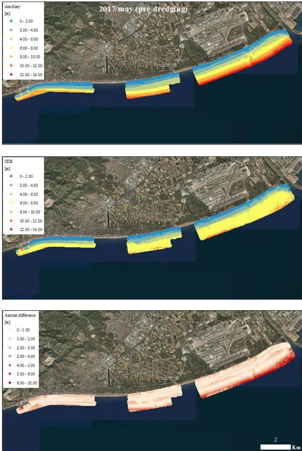
**Figure 18: Measured (23/may - upper panel) and satellite-based bathymetry (23/may - mid panel) from 2017 and the absolute difference between both (lower panel).**
