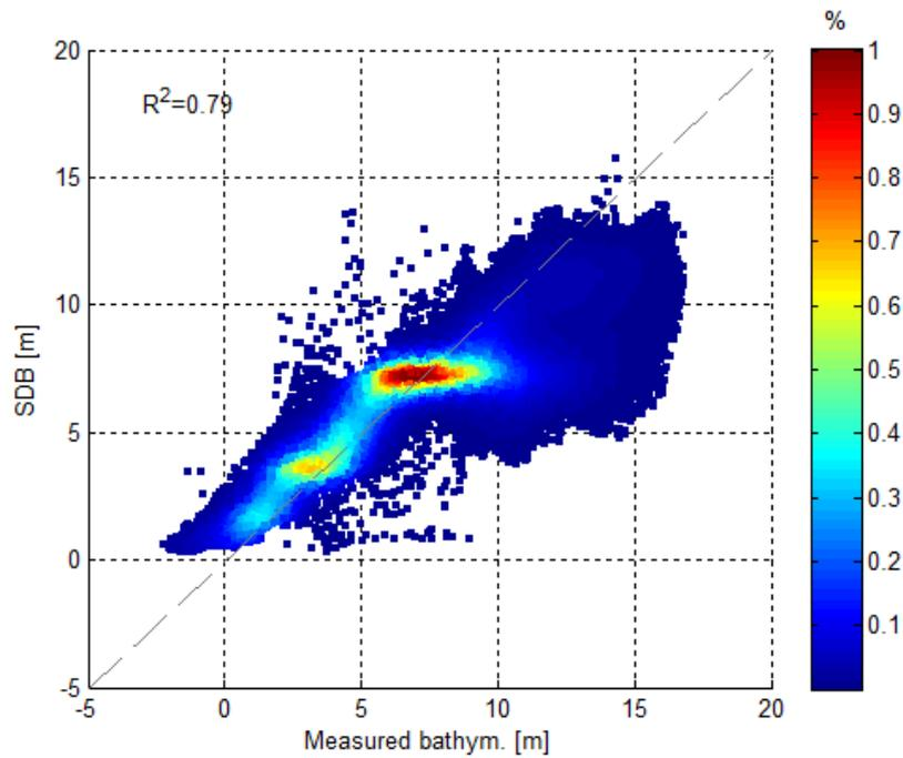
**Figure 20: Scatterplot between measured and satellite derived bathymetry. The scale of colors indicate points' density, in percent.**
