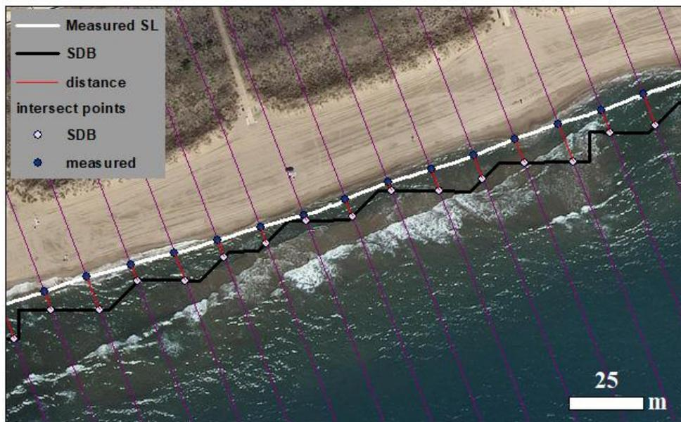
**Figure 12: Intersect points and distance between measured and satellite-based shorelines.**
