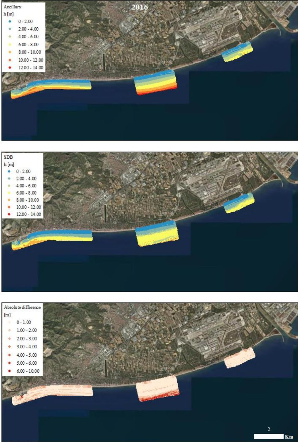
**Figure 17: Measured (01/jun - upper panel) and satellite-based bathymetry (07/jun - mid panel) from 2016 and the absolute difference between both (lower panel).**
