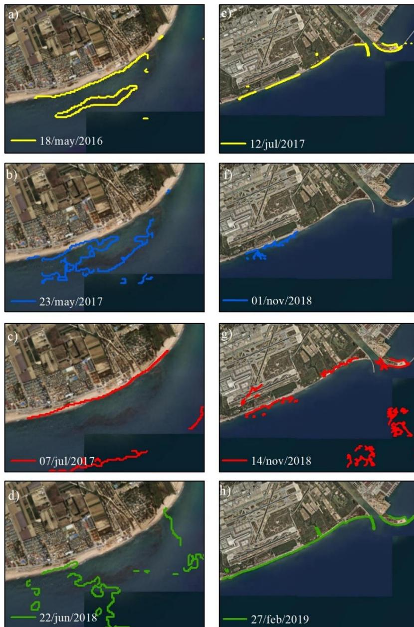
**Figure 8: Examples of inconsistencies verified in satellite-derived shorelines in both validation sites: Malgrat (left panels) and Barcelona (right panels).**
