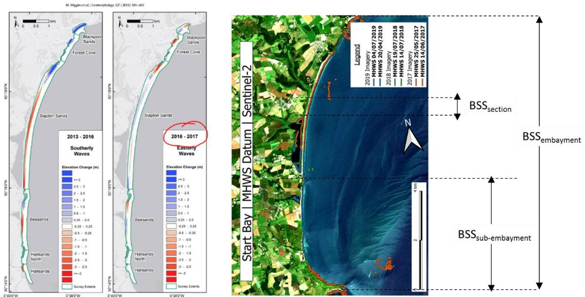
**Figure 4: Illustration of baseline data and EO products for Start Bay, UK. The left and central panel shows the topo-bathymetric changes observed at Start Bay for two time periods (2013-2016 & 2016-2017) (from Wiggings et al. (2019)). The beach rotates, clockwise or counter-clock-wise in function of the direction of the dominant highest waves. The right panel shows the EO derived MHW lines for different dates.**
