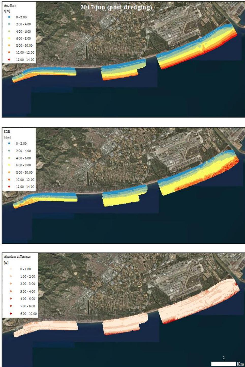
**Figure 19: Measured (13/jun - upper panel) and satellite-based bathymetry (12/jun - mid panel) from 2017 and the absolute difference between both (lower panel).**
