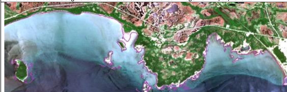
Continuous waterline segment at land-water interface from S2 image from 11/07/2019
