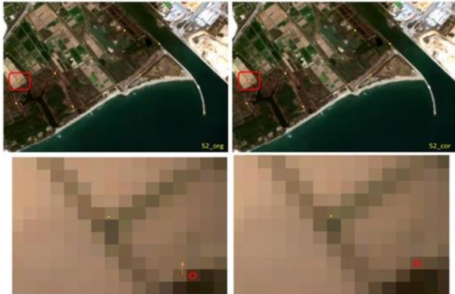
Figure 1.1:Co-registration shift of a Barcelona product (original product on the left, co-registered product on the right). The tie point (yellow dot) uses an agricultural field boundary. The pixel shift is shown in the lower right of the images (red circle).
