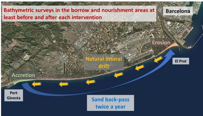
Figure 2.2 Sand back-pass performed in Barcelona beach
