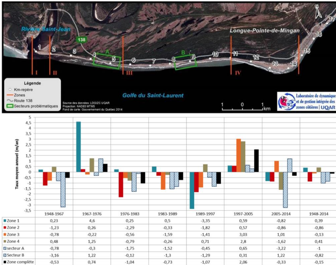
Figure 2.2: Coastal Evolution for 4 sub-coastal area (see transects), only for areas A and B and for the whole area (adapted from Corriveau et al., 2016)
