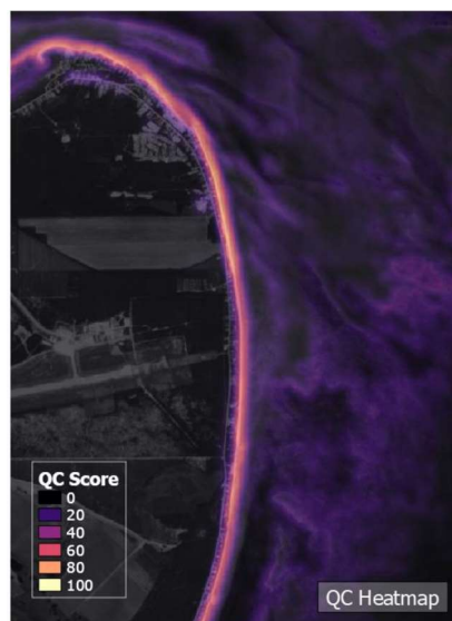
Figure 2.10: External quality control – darker colours representing noise, and the bright line around the coast showing the density of waterlines where we would expect to detect them.
