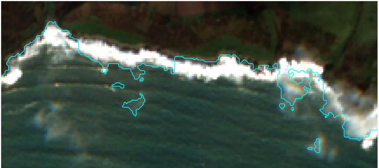
Figure 1.4: Waterline detected by the V3 processor in Start Bay (15/01/2020)
