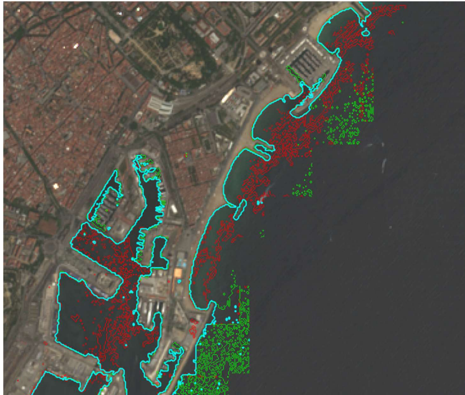
Figure 2.7: Waterline performance differences for different spectral indices: NDVI (red), GNDVI (green), BNDVI (cyan). Barcelona (tile: 31TDF), 02/07/2019.
