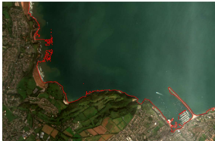
Figure 1.3: Noise contained in an otherwise accurate waterline in Start Bay (07/10/2018)
