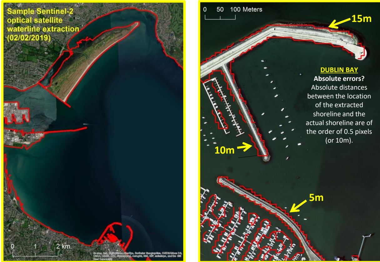
Figure 2.1: Location of Dunleary within Dublin bay, and a selection of Waterline positional accuracy measurements observed within a Dublin (Dunleary) Sentinel-2 Waterline (02/02/2019)
