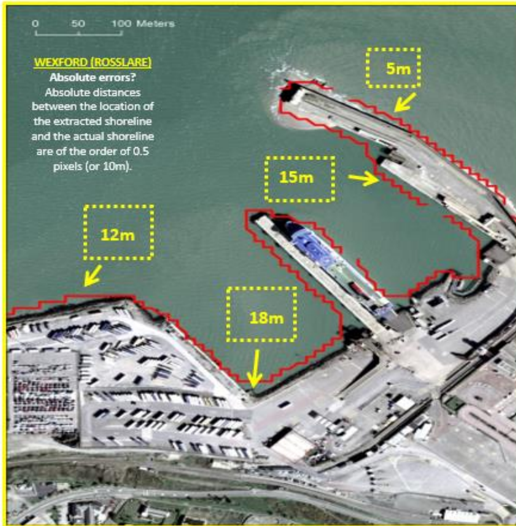
Figure 2.2: Positional accuracy measurements within a Wexford (Rosslare) Sentinel-2 Waterline
