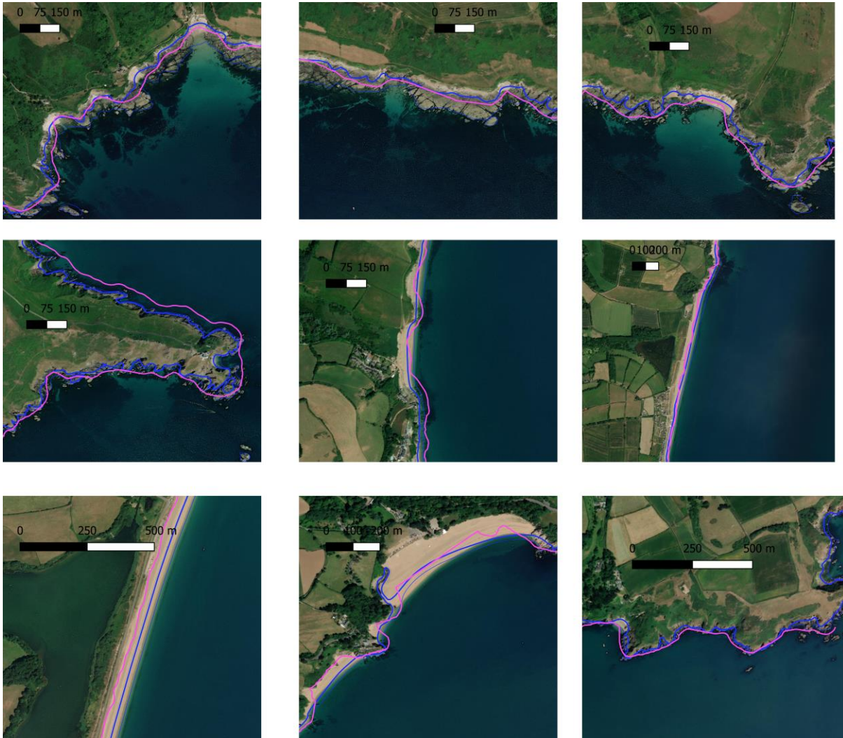
Figure 3.16.- Comparison of WL-SAR (magenta) vs OS HWM (thick blue) and LWM (thin blue) tidal boundaries (Nov 2019) for Start Bay study area. WL is for date 20 th Oct 2019 (Descending image, polarization VH). Product file name: S1B_IW_GRDH_1SDV_20191020T062303_20191020T062328_018555_022F5A_2372_QC_HM_CLASS_Good.geojson
