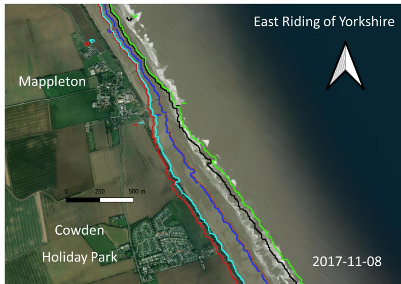
Figure 1.6.- Waterline (WL) is converted to different shorelines (SL) at different user-defined datum elevations (HAT, MHWS, MSL, MLWS, LAT). Example of shorelines produced for a segment of coast of beach backed type, by soft cliff at East Riding of Yorkshire region. Aerial imagery in the background shown for reference and taken at different date and time than shorelines.
