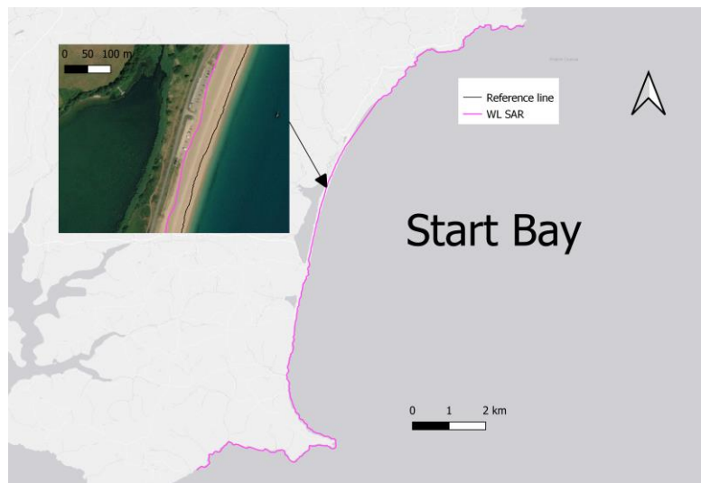
Figure 1.5.- Example of Waterline (magenta line) derived from SAR data (S1) for Start Bay. Also shown the reference line used by the service provider to assess the quality of the line. Product filename:
