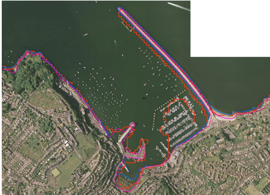
Figure 3.5.- Comparison of OS HWM and LWM and Landsat 8 waterline for Brixham Harbour.
