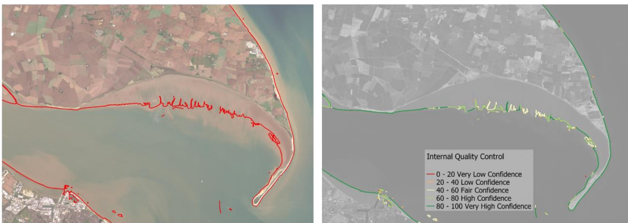
Figure 1.4.- Example of Waterline product produced for Humber estuary area. Left: waterline location over an aerial image of the area taken at different date and time than the WL. Right: line location colour coded using the quality flags metadata provided.
