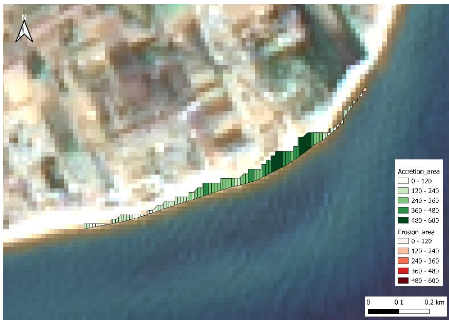
Figure 2.20: Time series result showing the beach renourishment between March and June 2015 in Malgrat beach, Torera Spain.
