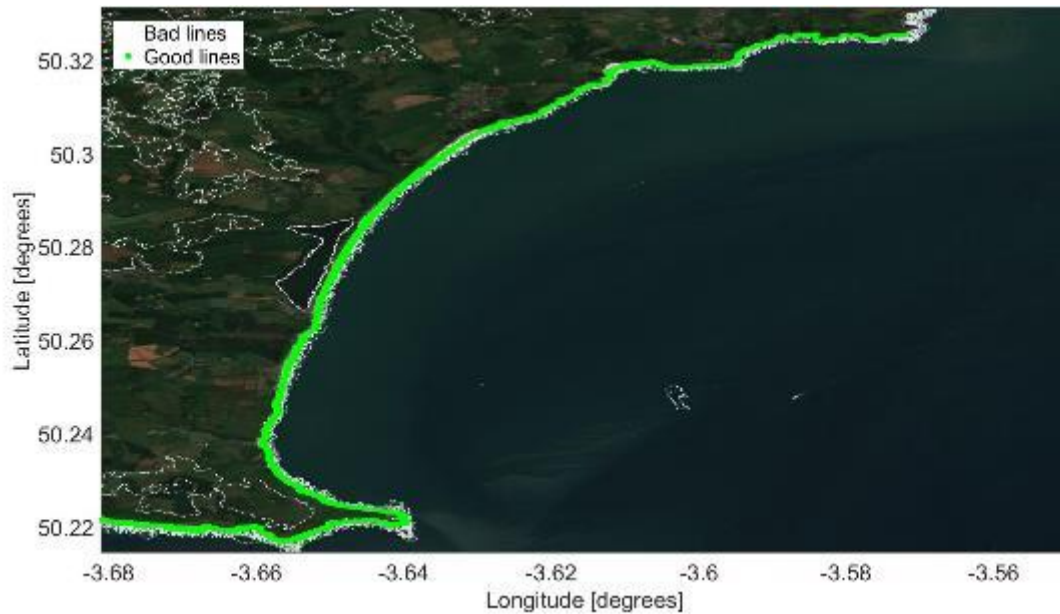
Figure 2.6: Waterlines generated from Sentinel 1 between 2014 and 2020 around Start Bay area. Green lines have been classified as “good” whereas the white ones are considered “bad” as the distance to the reference and the density are below the thresholds (50 meters and 2%)
