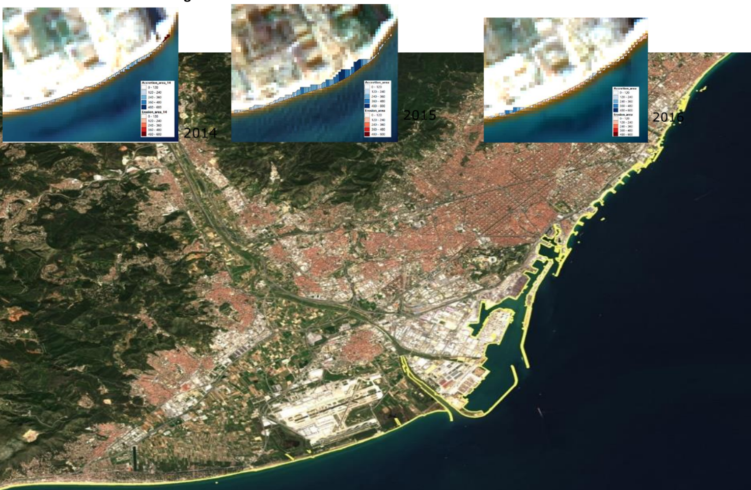
Mean annual shoreline change derived from the differences in individual shoreline extents.
